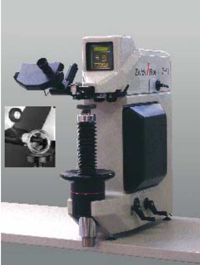
Zwick/ZHU 187.5 Universal Hardness Tester
