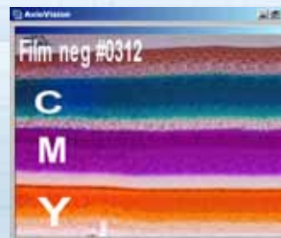
Cross-section of film with color layers indicated.
