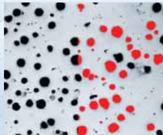
Cast iron evaluation with AxiVision Graphite
