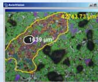
Clinker material in transmitted light, phase determination.
