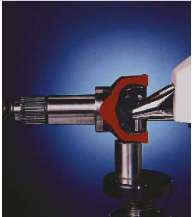
Indenter holder to enable hardness tests on measuring locations that are hard to gain access to
